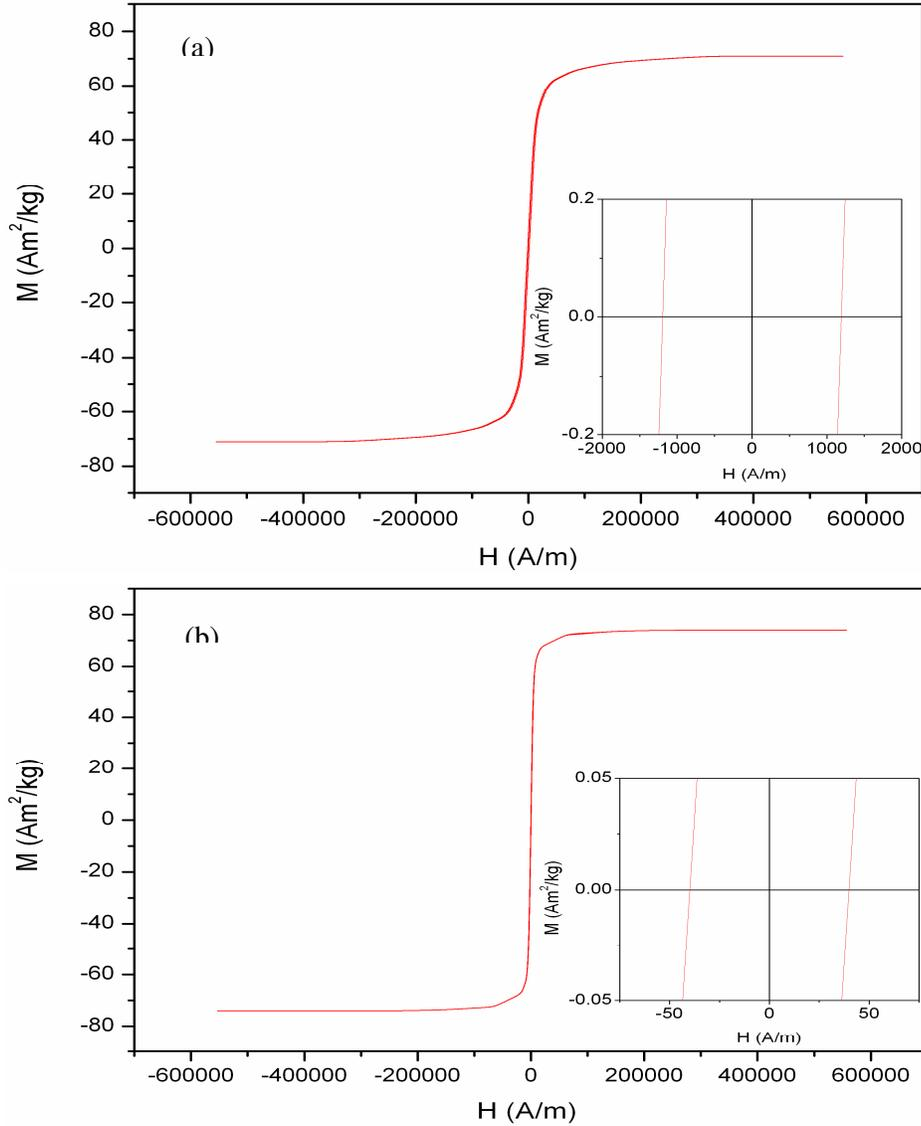
Fig.2. Hysteresis loops of as-cast (a) and splat-quenched (b) samples of  $\text{Fe}_{25}\text{B}_{17.5}\text{Co}_{21.35}\text{Nb}_{3.65}\text{Ni}_{25}\text{Si}_{7.5}$  HEA.
