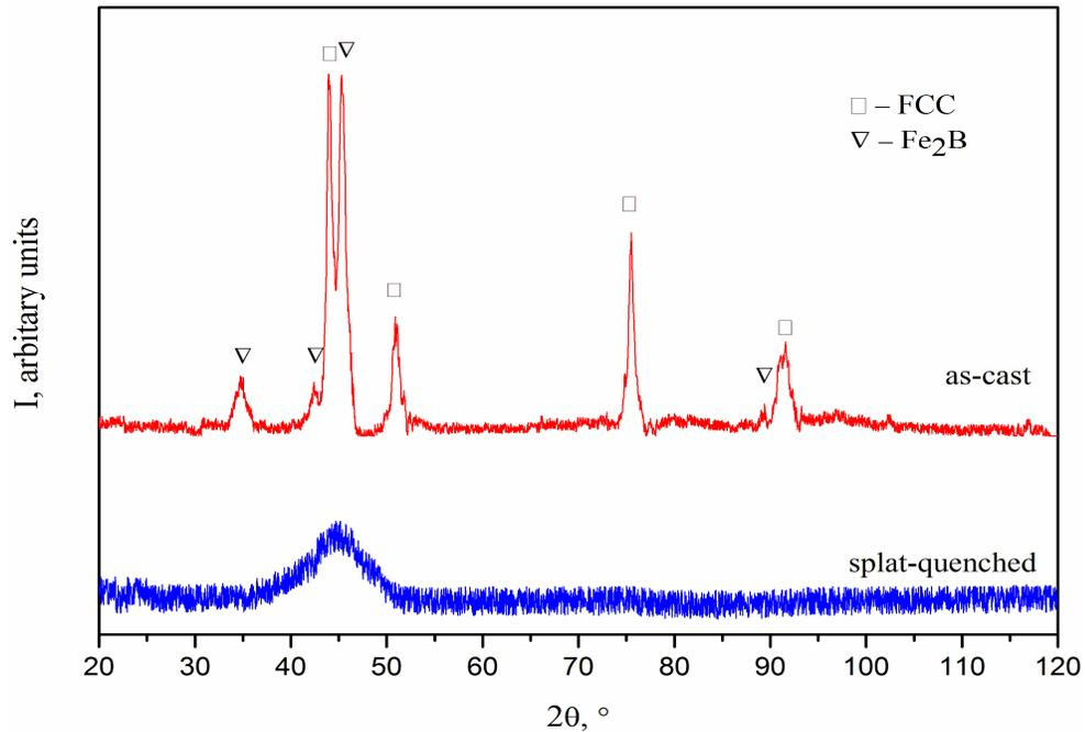
Fig.1. XRD patterns of as-cast ingots and splat-quenched films of  $\text{Fe}_{25}\text{B}_{17.5}\text{Co}_{21.35}\text{Nb}_{3.65}\text{Ni}_{25}\text{Si}_{7.5}$  HEA.
