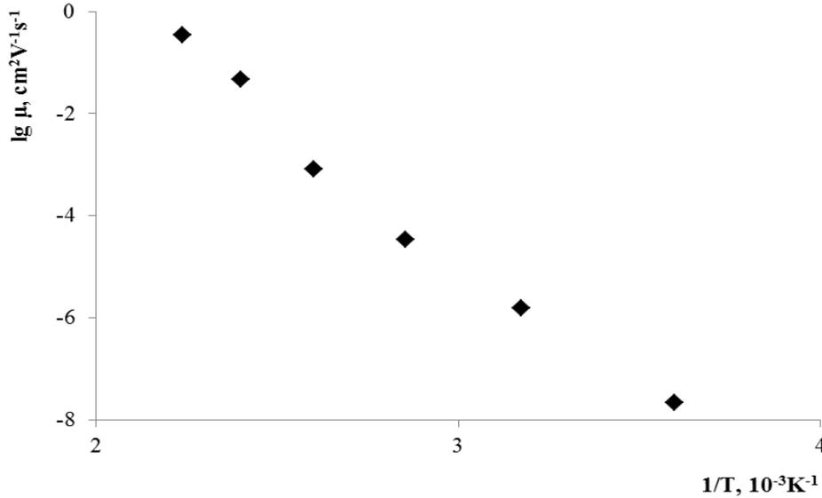
Fig. 3. The temperature dependence of the mobility of  $\text{Bi}_2\text{TeO}_5:\text{Fe}$  single crystals.
