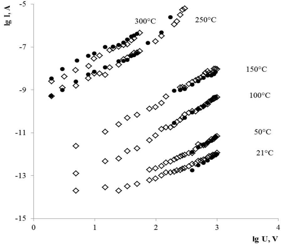
**Fig. 2.** The current-voltage characteristics at different temperatures of  $\text{Bi}_2\text{TeO}_5\text{:Fe}$  single crystals. White markers – forward process, black markers – backward process.
