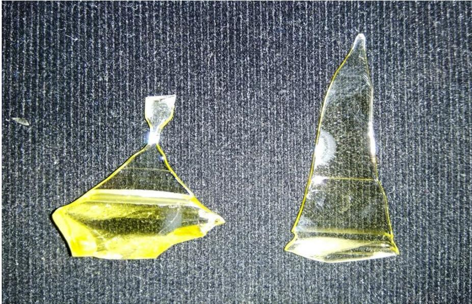
Fig. 1. Bismuth tellurite single crystal doped by  $\text{Fe}_2\text{O}_3$  grown by Czochralski method.
