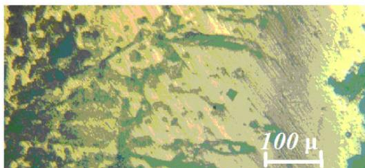
Fig. 1. Microstructure of titanium sample after the TT in the boron-containing medium,  $\times 1000$
