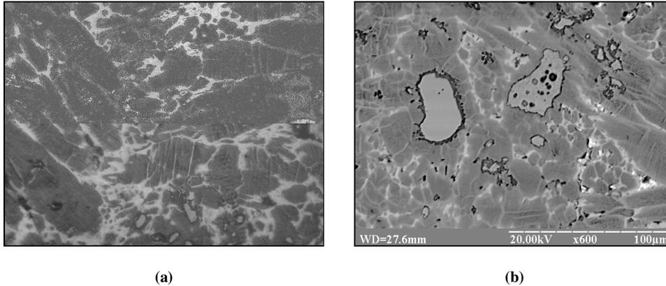
Fig. 1. Microstructure of  $\text{Al}_{65}\text{Co}_{20}\text{Cu}_{15}$  alloy: a – optical micrograph,  $\times 400$ ; b – SEM micrograph,  $\times 600$ .
