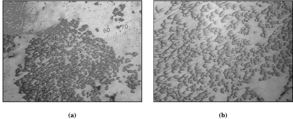
**Fig. 2. Microstructure of composites reinforced with Al-Co-Cu particles infiltrated by : a – JL62 alloy,  $\times 400$ ; b – БрОЦ 10-2 alloy,  $\times 600$ .**
