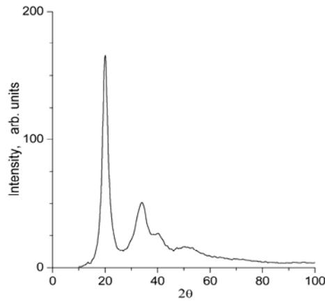
Fig. 1. Mo  $K_{\alpha}$  X-ray diffraction pattern of initial microwire.
