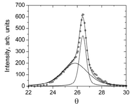
Fig. 4. Co  $K_{\alpha}$  X-ray diffraction pattern of microwires treated at 550 °C (5 min).
