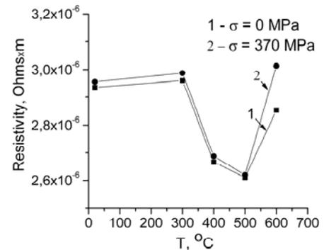
Fig. 3. The temperature dependence of the resistivity of microwires.
