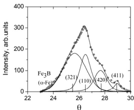
**Fig. 5. Co  $K_{\alpha}$  X-ray diffraction pattern of microwires treated at 550 °C (5 min) under stress 110 MPa.**
