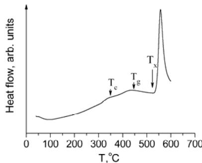
Fig. 2. The differential scanning calorimeter curve for microwires.
